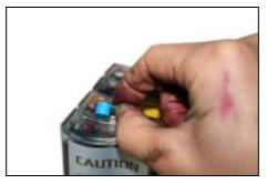
Pull out the small rubber plug from the air hole as the picture shown above.
